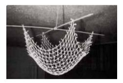
Heinz Isler, hanging models and draped fabrics, sprayed with water and frozen lead to almost immaterial shell structures.
